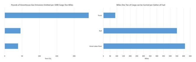
FIGURE 30—CARBON DIOXIDE (CO<sup>2</sup>) EMISSIONS AND GALLONS OF FUEL USED TO MOVE CARGO
