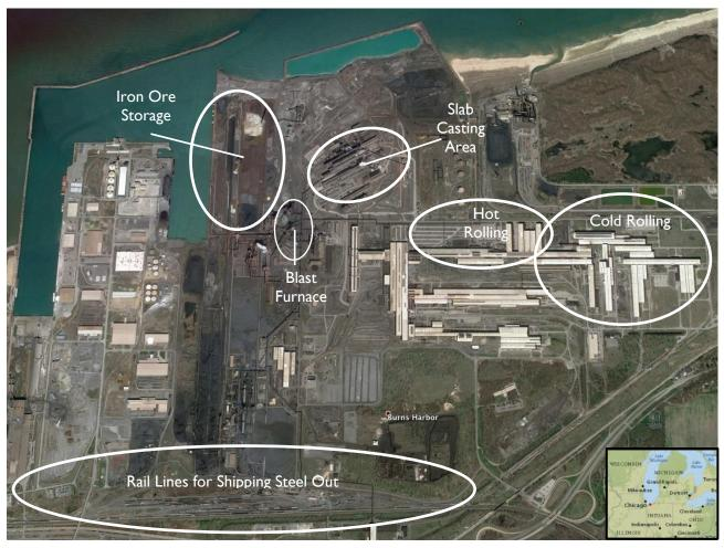
FIGURE 28—BURNS HARBOR STEEL MILL
