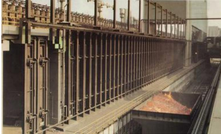
**FIGURE 5—COKE BATTERY SHOWING THE SIDE-BY-SIDE OVENS AND A RAILROAD CAR OF INCANDESCENT COKE<sup>14</sup>**
