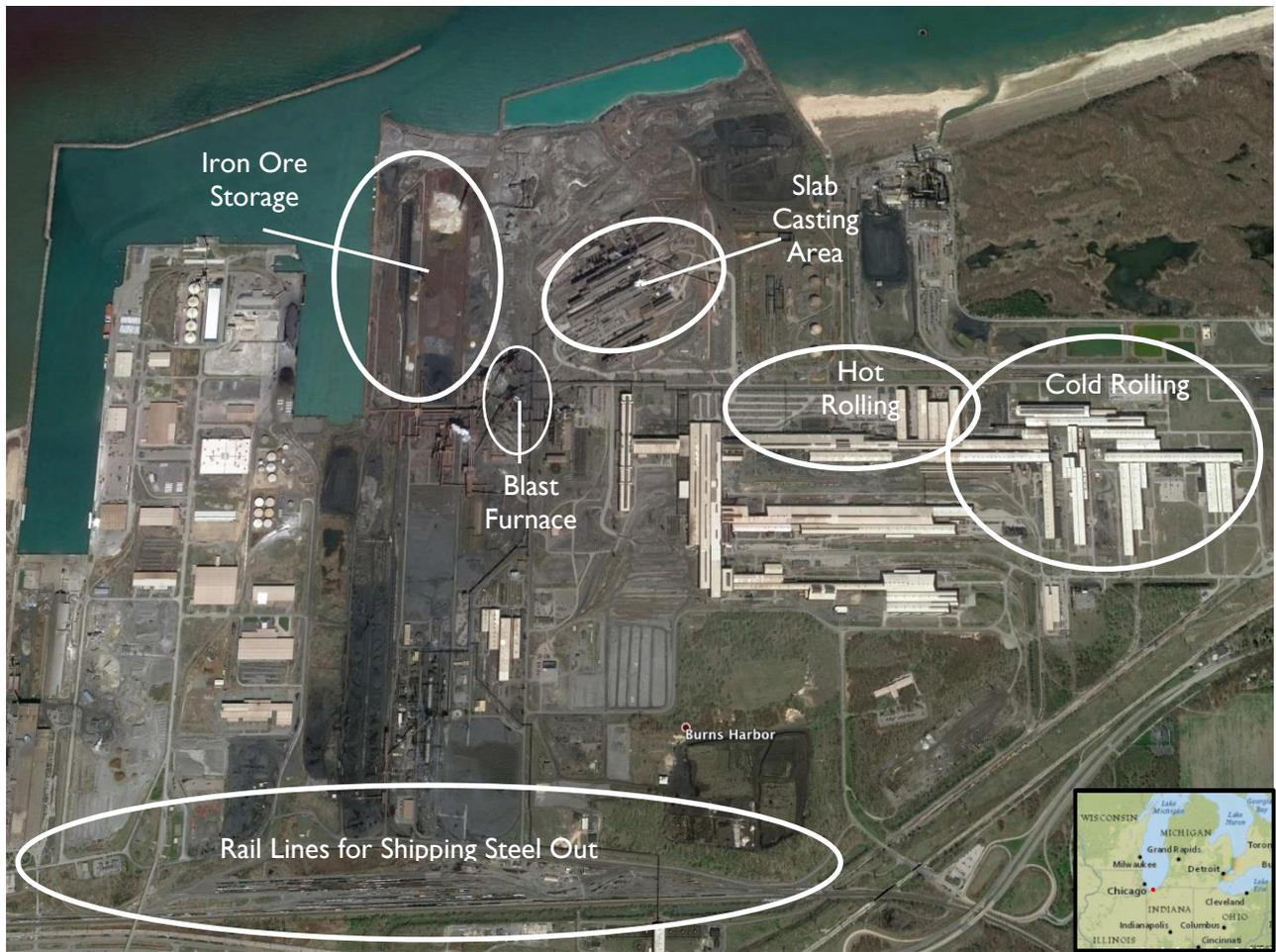
**FIGURE 28—BURNS HARBOR STEEL MILL**
